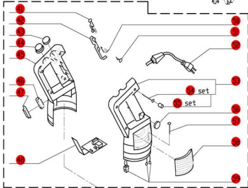
If replacing internal parts within dashed lines, order a set of replacement screw caps, part # MP29544.
